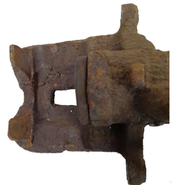
3. Excessive disc wear to casting
