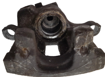
5. Missing components i.e. No levers, springs, pistons or internal hardware
