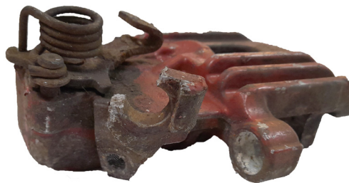
2. Damaged, cracked or broken castings
